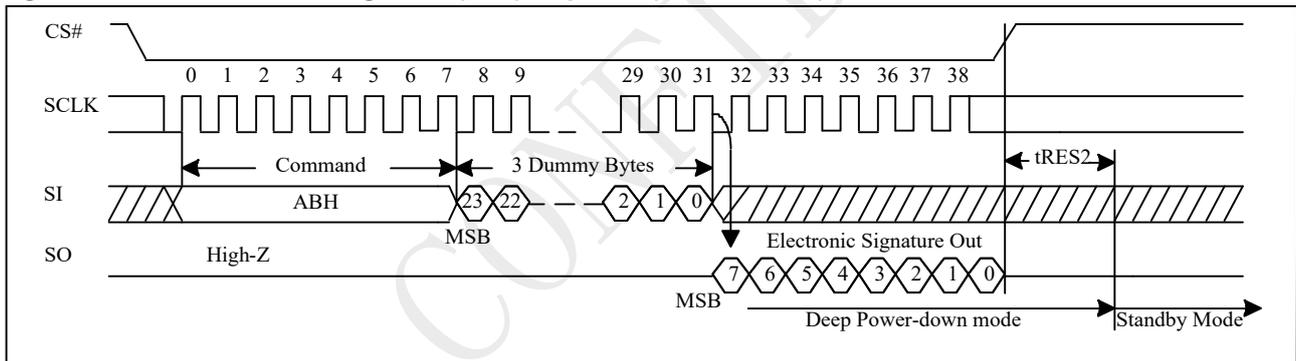
**Figure 10-42a Read Electronic Signature (RES) Sequence (QPI)**
