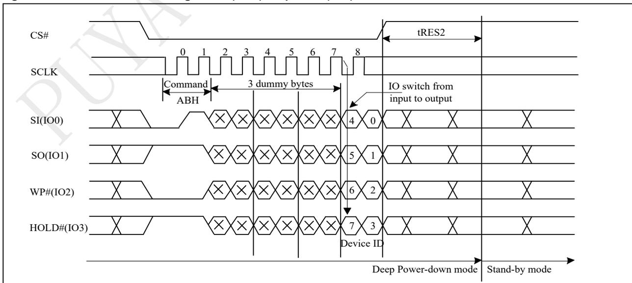
**Figure 10-42b Release from Deep Power-down (RDP) Sequence (Command AB)**
