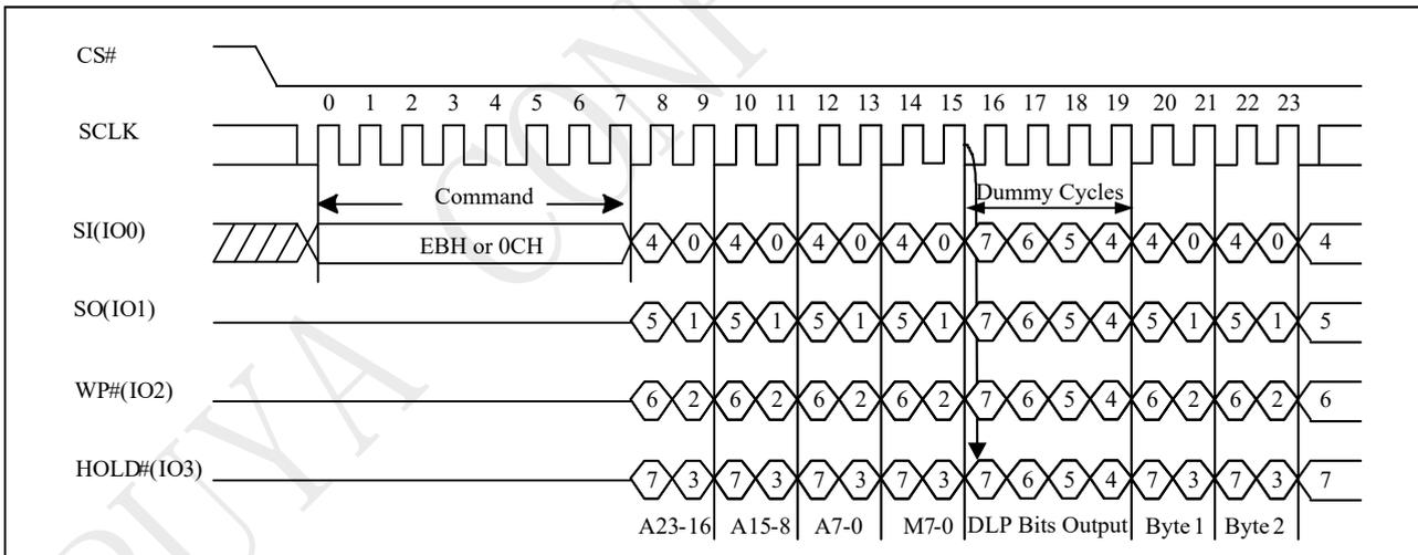
Figure 10-23d 4IO Read and Burst Read with DLP bits output Sequence in QPI mode
