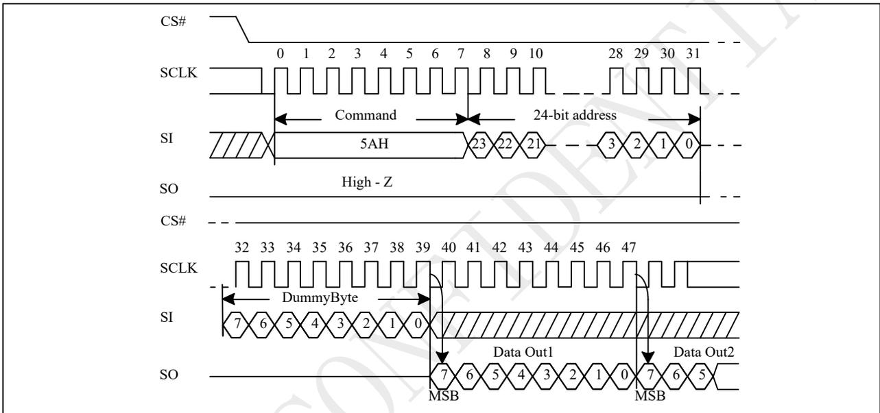
**Figure 10-58a Read Serial Flash Discoverable Parameter (RDSFDP) Sequence(QPI)**
