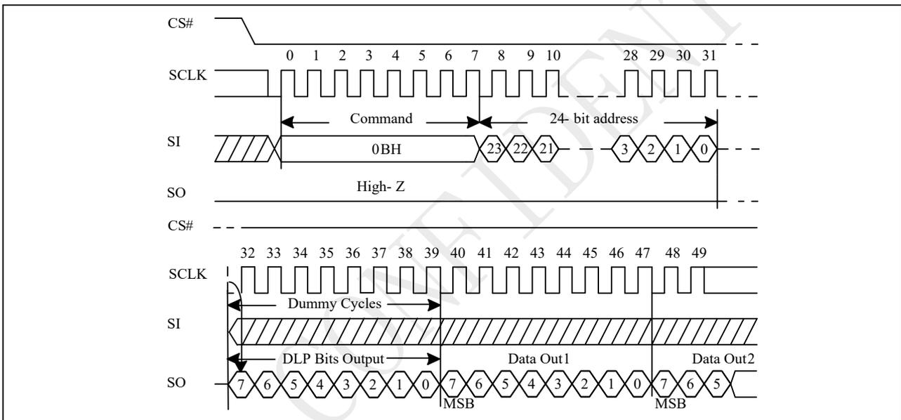
**Figure 10-23a Dual Read with DLP bits output Sequence**
