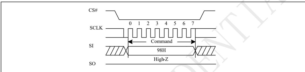
**Figure 10-54a Global Block Unlock(QPI)**
