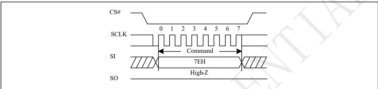
**Figure 10-53a Global Block Lock(QPI)**
