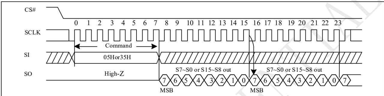
**Figure 10-5a Read Status Register (RDSR) Sequence (QPI)**
