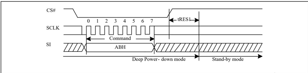
**Figure 10-42c Release from Deep Power-down (RDP) Sequence (QPI)**
